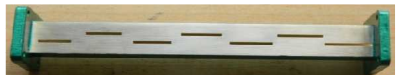
Fig. 2. Top view of fabricated 7-element longitudinal log periodic slot array antenna with flange.
